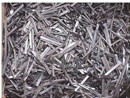
Scarf chopped in the Sweed TS450 is safely and easily compacted—Approximately 2000 linear feet of chopped scarf easily fits into a 12" x 10" x 4" box.
