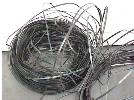
Scarf from a winder is dangerous, bulky and not easy to handle.
