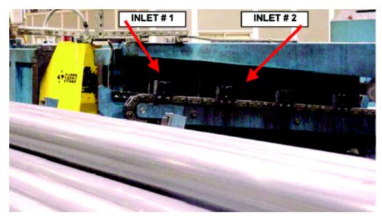
Two tubes are processed at the same time. A blast of water followed by compressed air delivers the ID scarf into the chopper. The ID scarf is chopped up into random lengths from 6 to 8 inches.
